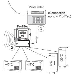
Chilling or freezing device with no-volt remote alarm contact
